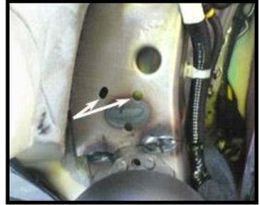
2. Using a 7/16" socket and the the two 1/4 "x 20 bolts and kep nuts supplied, install the bracket to the mounting holes. The holes of the bracket should be at the bottom and the stop pin should be at the top.
